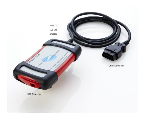
There are three main parts to the device and these are shown on the picture above.
