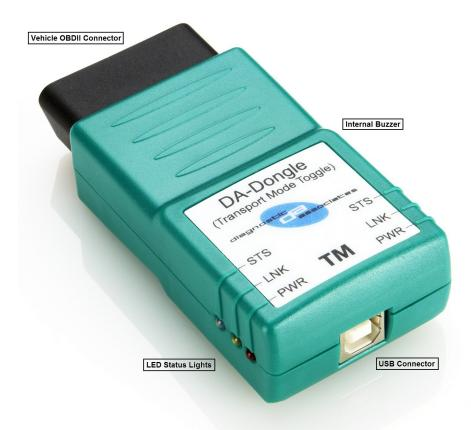
There are four main parts to the device and these are shown on the picture above.
