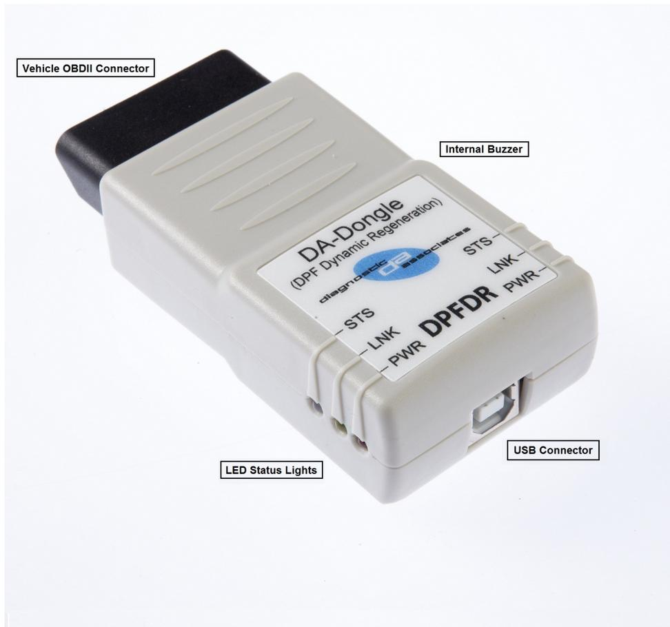
There are four main parts to the device and these are shown on the picture above.
